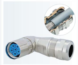
An integrated metalized EMI clamping insert grounds to the braid signifficantly simplifying the assembly of the elbow connector.
