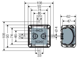
2x Ø6-15 mm 2xM20 2x Ø6-15 mm 2x Ø6-15 mm Box walls 2xM20 2xM20 L<sub>1x</sub> Ø6-15 mm-1xM20
