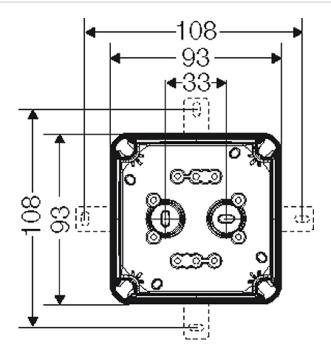
2x Ø6-15 mm 2xM20 2x Ø6-15 mm 2x Ø6-15 mm 2xM20 2xM20 L<sub>1x</sub> Ø6-15 mm 1xM20
