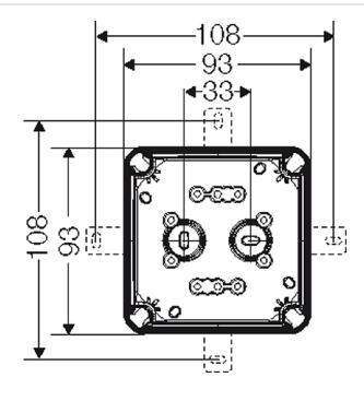
2xM20 2x Ø6-15 mm 2x Ø6-15 mm 2xM20 2xM20 L<sub>1x</sub> Ø6-15 mm-
