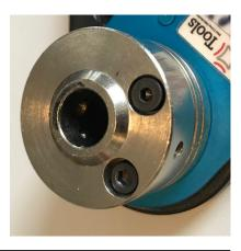
Step 4: Insert the locator-bolt. The groove will snap in when the locator is in position.
