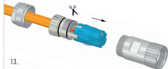
**⚠** Make sure, that the braided shield doesn't contact the rear O-ring
